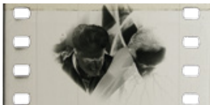
Visible sparks: Detail of a frame from the camera negative with imprinted marks from static electricity
