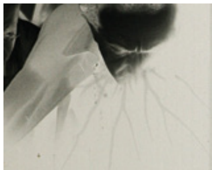
Visible sparks: Detail of a frame from the camera negative with imprinted marks from static electricity
